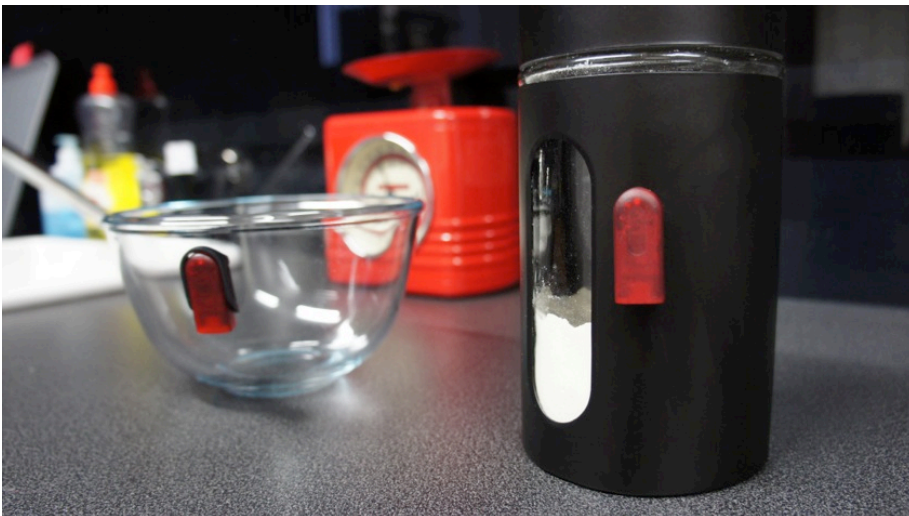
Figure 1: Digital sensors attached to cooking equipment
